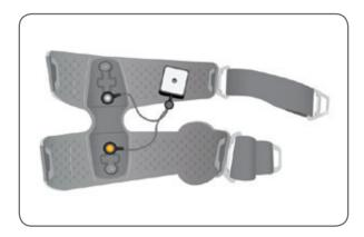
Figure 13-2: Tester Connected to Thigh Cuff
